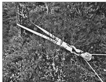
Figure 7 refers to an illustration of one of the most popular rigging methods. In this situation, a winch-mounted vehicle is being used with a nylon strap around a tree.
