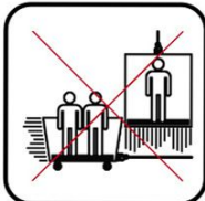
Under no circumstances utilize a Winch to lift and/or move People or Animals
